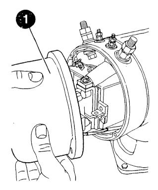
Unfasten cover plate bolts and detach cover plate (1) with sealing plate (2).
